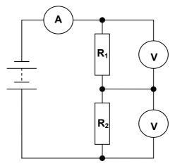
The potential difference  $V_1$  across resistor  $R_1$ , the potential difference  $V_2$  across resistor  $R_2$ , and the potential difference  $V_t$  across the power supply are related by the equations
